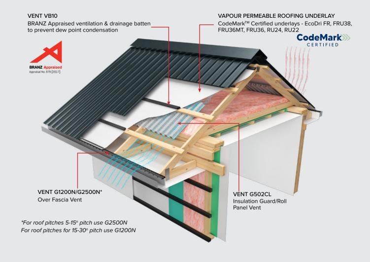
Products must be used in combination as recognised in DriSpace technical details to ensure that essential calculated, continuous, unimpeded passive ventilation is achieved.
