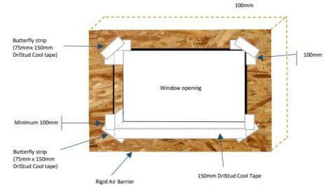
3. On the two upper corners cut the Cool Tape to required length allowing a minimum of 100mm for the jamb. Apply to the interior face of the opening, along the length of the lintel and down the jamb. Cut the overhanging tape at each corner, fold and secure, then apply a 75mm by 150mm butterfly seal over top at a 45° angle. Ensure the tape is pressed firmly onto substrate and applied tightly into all corners.
